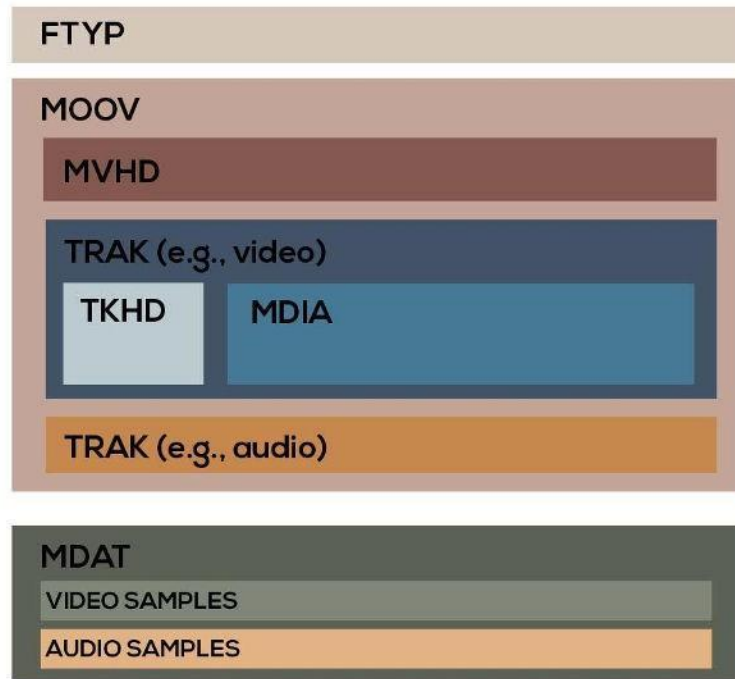
Figure 1. An illustration of some of the components that constitute an ISO Base Media File Format (e.g., MP4, MOV, 3GP) video file structure. (Image Credit: SWGDE)
