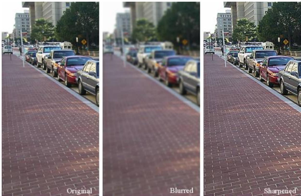
Figure 1. This example illustrates the effects of linear filtering. Left: original image; Middle: blurred image; Right: sharpened image.
