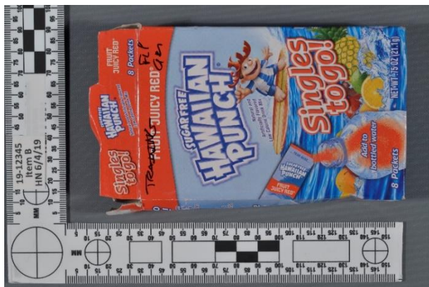
(C) Scale is at a lower plane than the item (appears smaller than actual size).
