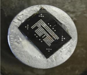
Figure 9 – Example of circuit board and solder mask removed
