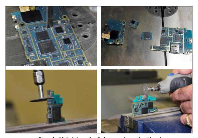
Figure 2 – Methods for cutting flash memory from a circuit board
