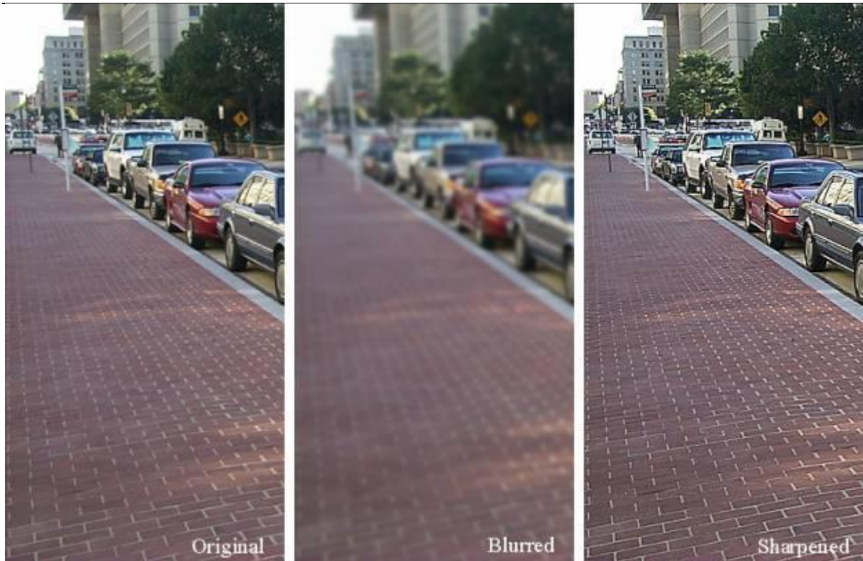
Figure 2. This example illustrates the effects of linear filtering. Left: original image; Middle: blurred image; Right: sharpened image.
