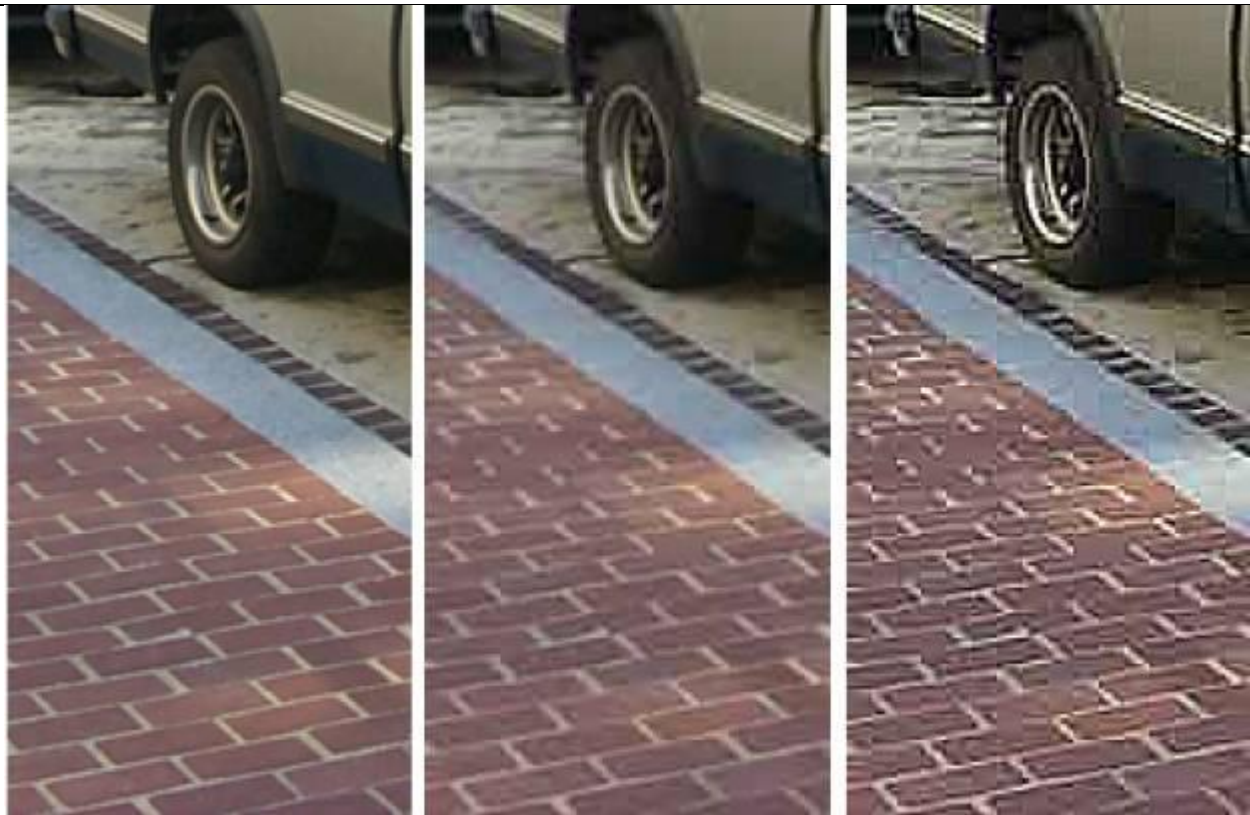
Figure 4. Left: original image; Middle: the result of JPEG compression (compression ratio = 15:1); Right: the result of edge enhancement after compression.
